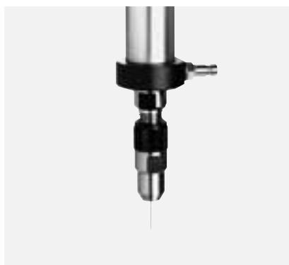
Reglus electrode holder with 20-mm- \varnothing shaft with rotating flushing connection (Type 350.20.E) or with internal flushing channel, flushing via the spindle (Type 350.20.I).
