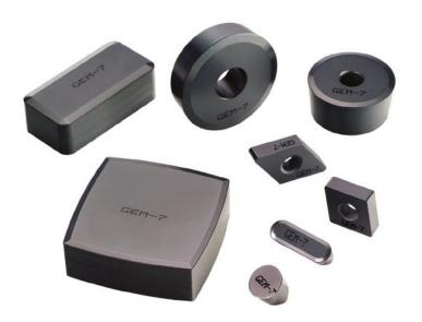
**GEM-7**<sup>™</sup> is an aluminum oxide and titanium carbide composite ceramic with a high degree of predictability in roll turning and hard alloy (up to 65 R/c) machining.
