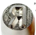
Positive impression punches have a negative readable face to produce a positive indent impression
