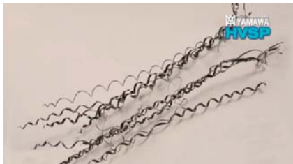
Ejected chips by large size taps
